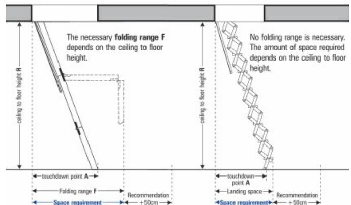
The specific space requirement (= folding range of the 3-section attic stairs and / or touchdown point with concertina loft ladders) depends on the ceiling to floor height. We recommend to add a further 50 cm of space for handling and a more comfortable use of the stairs.
